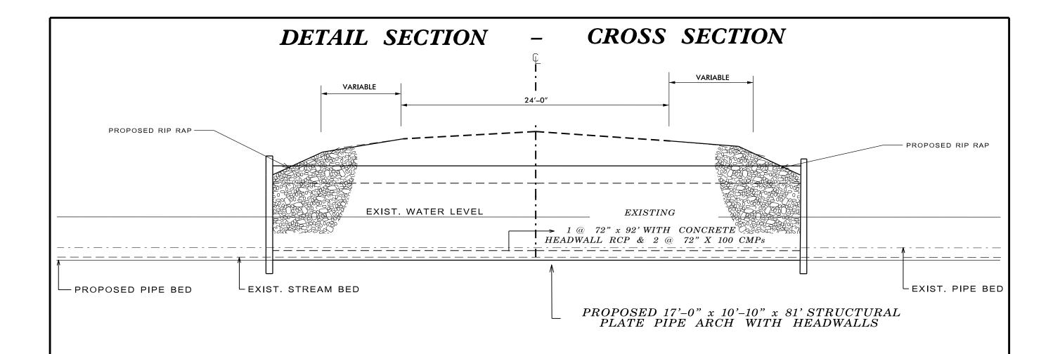
NOTES: \* PROPOSED 17'-0" X 10'-10" X 81' ALUMINUM STRUCTURAL PLATE PIPE ARCH TO BE BURIED 1.0' BELOW EXISTING STREAM BED
